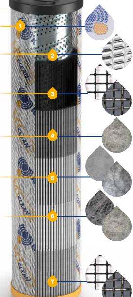
External metal mesh support for protection of the filtration medias from flow and pressure fluctuations and also to protect the integrity of the element's pleated structure.
