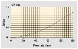
The curves are plotted using mineral oil with density of 0.86 kg/dm $^3$  in compliance with ISO 3968.  $\Delta p$  varies proportionally with density.
