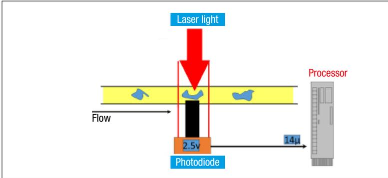
As the particle passes through the laser beam, the loss of light is directly proportional to the size of the particle
