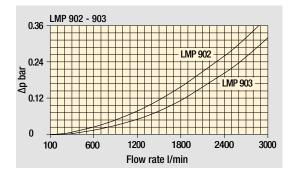
Bypass valve pressure drop
