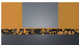
CONTAMINATION IN PRESENCE OF LARGE TOLERANCES
